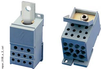
IP20 direct or cable connection distribution blocks which can be clipped onto a symmetric DIN rail.
